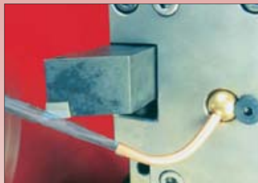
LolliPop nozzle shown installed in lathe turret.
