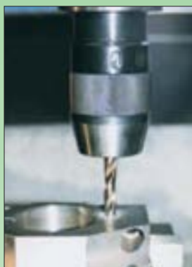
1 Drill coolant passage, leaving reaming allowance.
