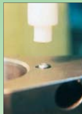
3 Press in JiffyJet until body is flush.
