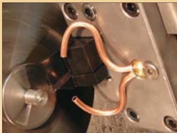
TwinPop nozzle shown installed in lathe turret.
