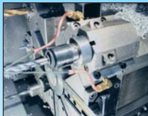
JetTubes shown on CNC turning center.
