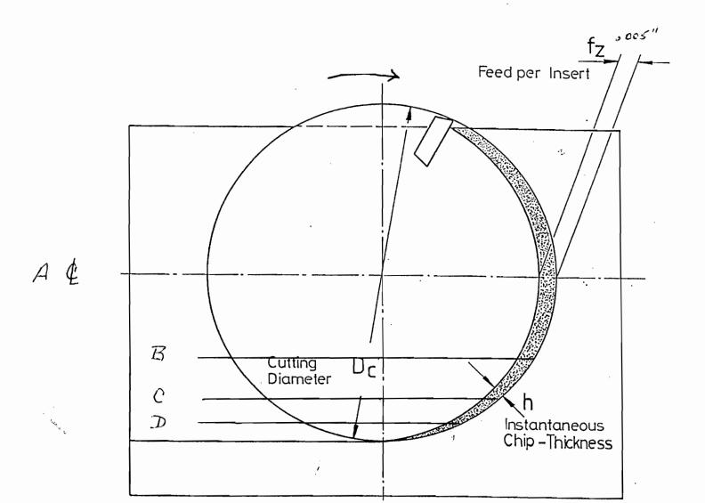
Each Milling Cutter, Milling Insert and Grade combination has a speed and feed range that it is designed to work best at. Once you know what feed is recommended for a particular cutter in the material you are cutting you can use this formula to maximize the performance of your tools and reduce your cycle time.
